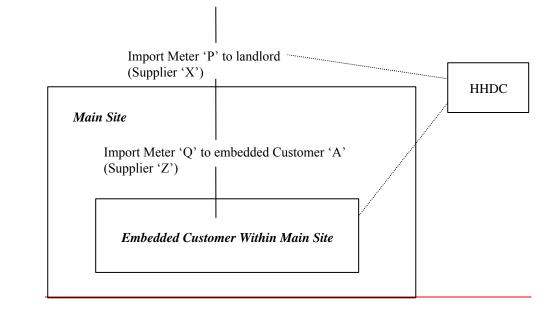
Landlord energy for Supplier 'X' = Meter 'P' Meter 'Q' HH data: 1 Import MSID Customer 'A' energy for Supplier 'Z' = Meter 'Q' HH data: 1 Import MSID No. of Import MSIDs = 2 (1 MSID for embedded customer and 1 for the landlord or Main site)
