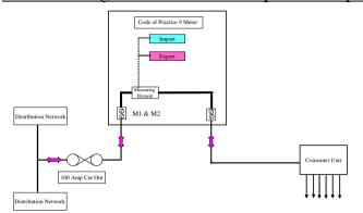
Schematic diagram of a combined Import and Export Meter – Whole Current
