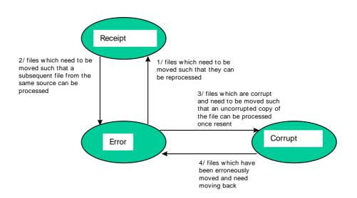
Note that the NHH Data Aggregator can also move files in the corrupt area back to the error area (flow 4). This is to rectify any incorrect movement of files to the corrupt area.
